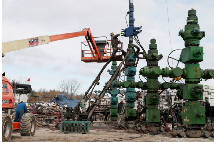
Figure 9. Blowout preventers (Christmas trees) at Marcellus shale formation, Camptown, Pennsylvania. Source: Southwestern Energy Co,
