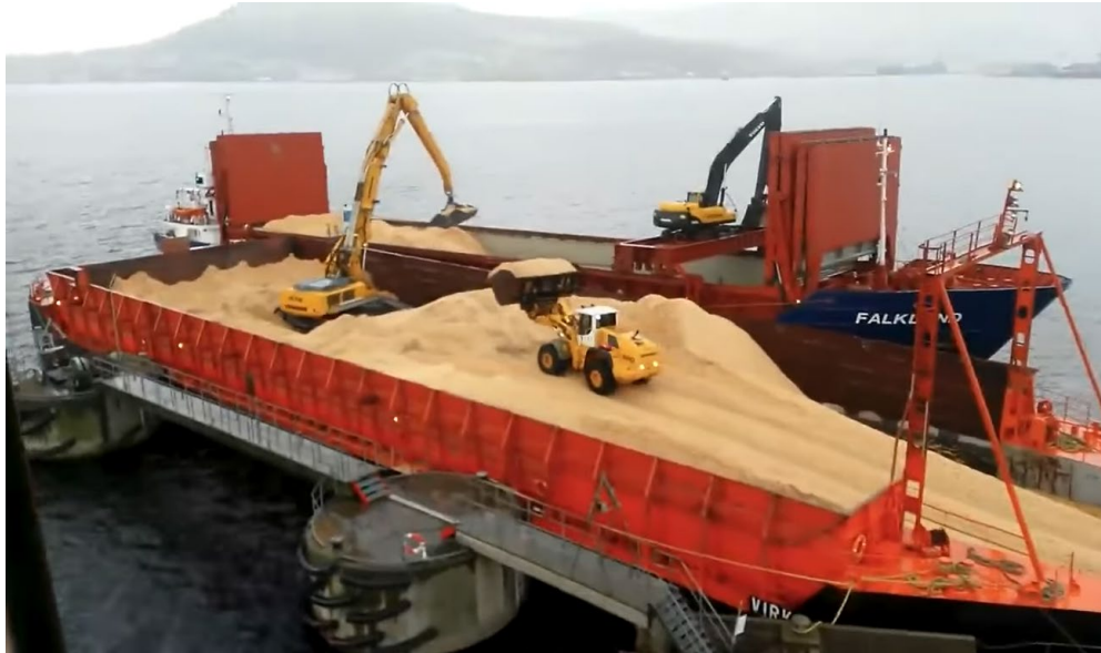
Figure 10. Loading cargo ship with wood pellets for export from barge.
