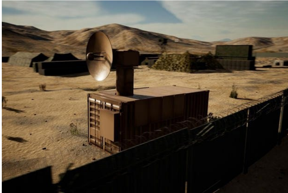
Figure 2. Air Force Research Laboratory's Tactical High-power Operational Responder, or THOR. THOR is a portable counter Unmanned Aircraft Systems UAS system capable of destroying swarms of drones at the speed-of-light, at long range, in its base defense mission. Source: Air Force Research Laboratory.
