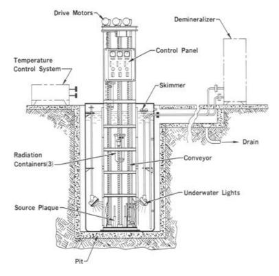
Figure 5. Water shielded irradiator configuration.
