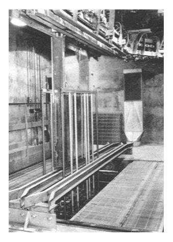
Figure 7. A conveyor rack passes between the raised Cobalt<sup>60</sup> rods at the USA Army Natick Labs food irradiator.
