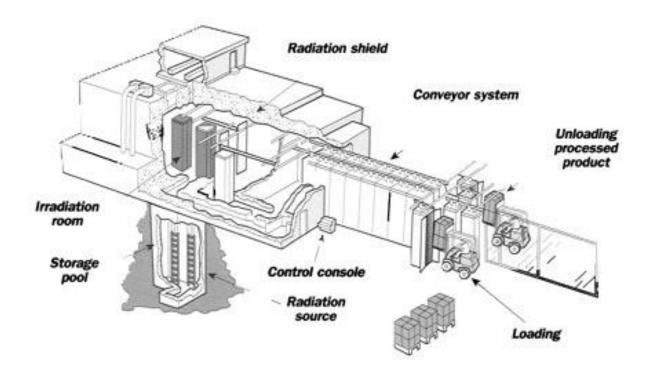
Figure 4. A typical Gamma Irradiation Facility.
