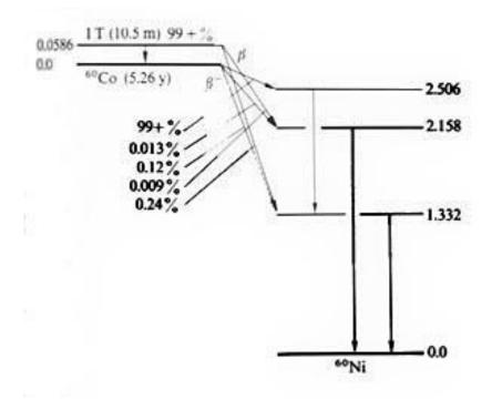
Figure 9. Decay Scheme of the Cobalt<sup>60</sup> isotope, showing the energies of gamma rays emission.
