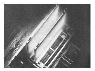
Figure 6. A Cobalt<sup>60</sup> irradiation source under water shielding emitting Cerenkóv radiation.
