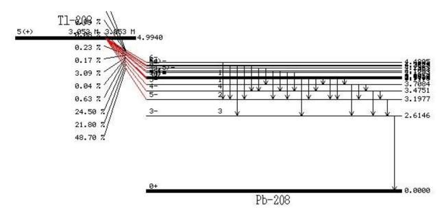
Figure 11. Gamma rays emissions from the Tl<sup>208</sup> isotope.
