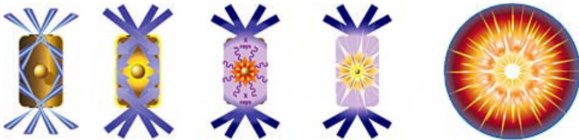
Figure 3. Indirect soft x-ray hohlraum drive compression of a fusion pellet.
