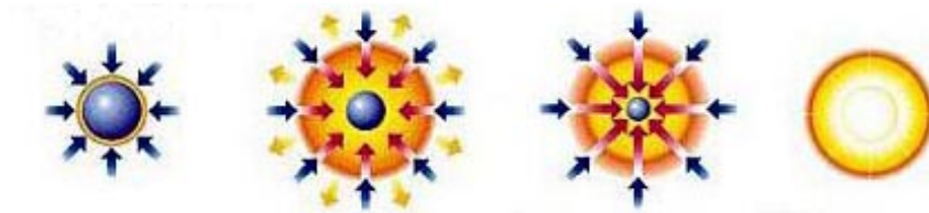
Figure 2. Direct laser drive compression of a fusion pellet.
