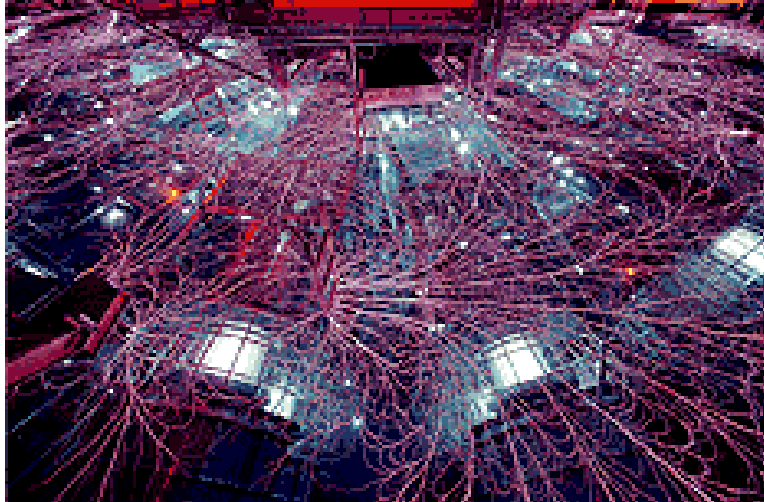
Figure 17. The Z-pinch facility at Sandia National Laboratory (SNL), showing electrical discharges in water along beam lines.
