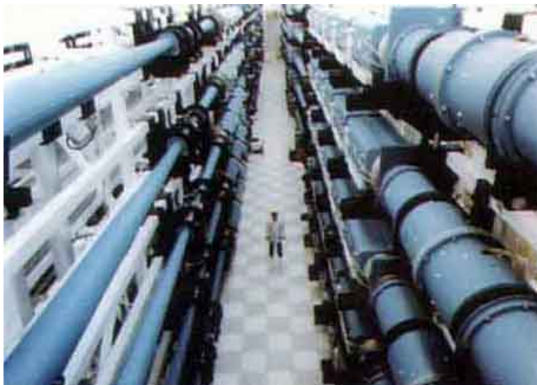
Figure 22. Laser beam lines of NOVA laser.
