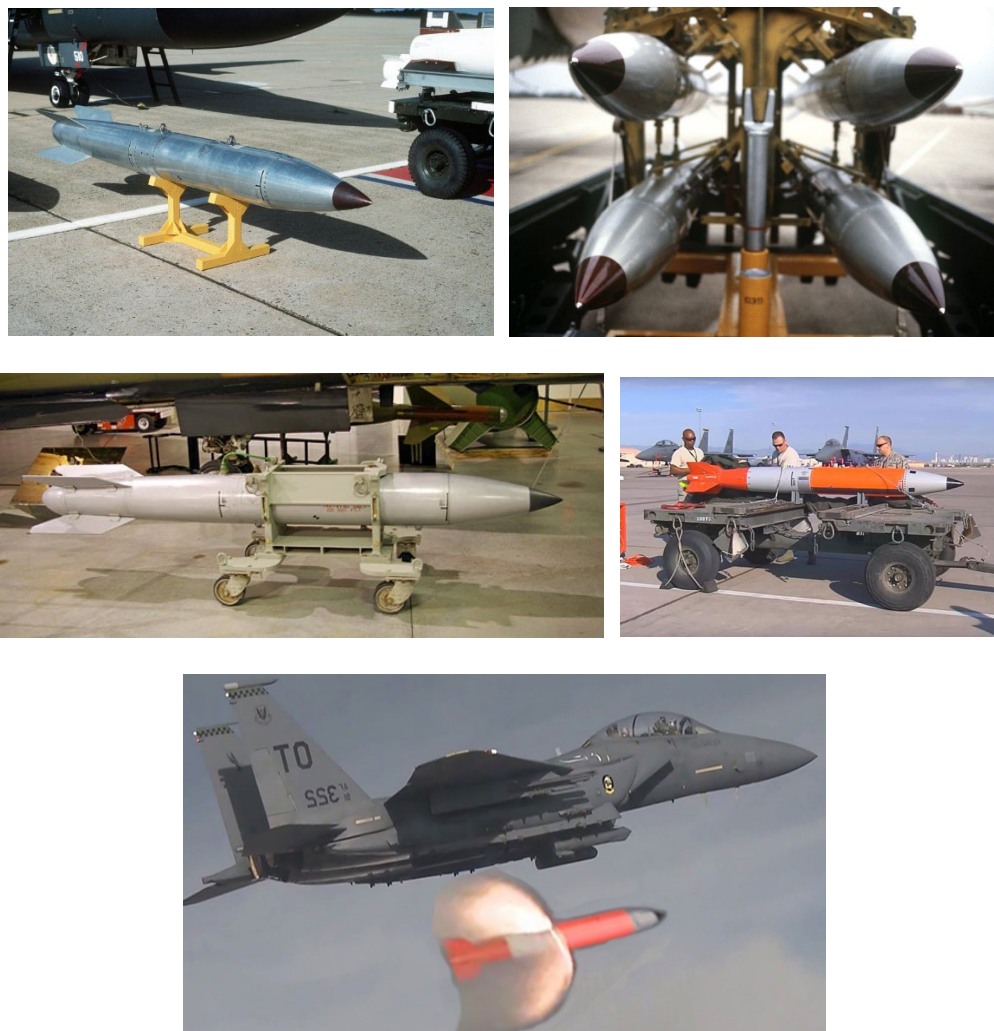
Figure 2. Thermonuclear B61-12 gravity high surety warhead equipped with tail fins and back rotational rockets for enhanced accuracy.
