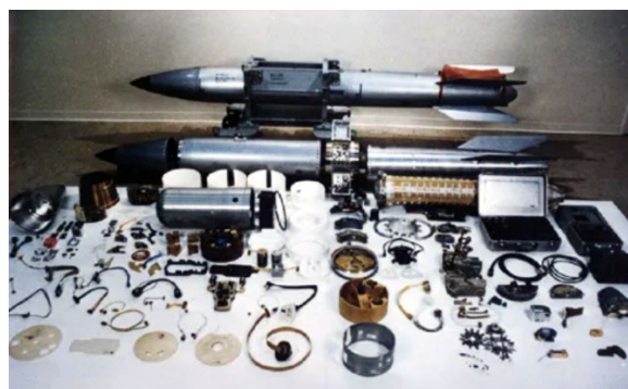
Figure 3. Three views of a B61 gravity bomb: assembled in the background, disassembled into its major subcomponents in the middle, and a display of some of the weapon's 5,919 parts in the foreground. The warhead fits inside the blunt-nosed silver canister sitting on the white cloth in front of the partially disassembled bomb. Source: LANL.
