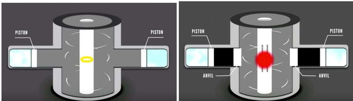
Figure 30. Magnetized target fusion. A plasma is injected into a liquid metal vortex then is compressed by steam-driven pistons.
