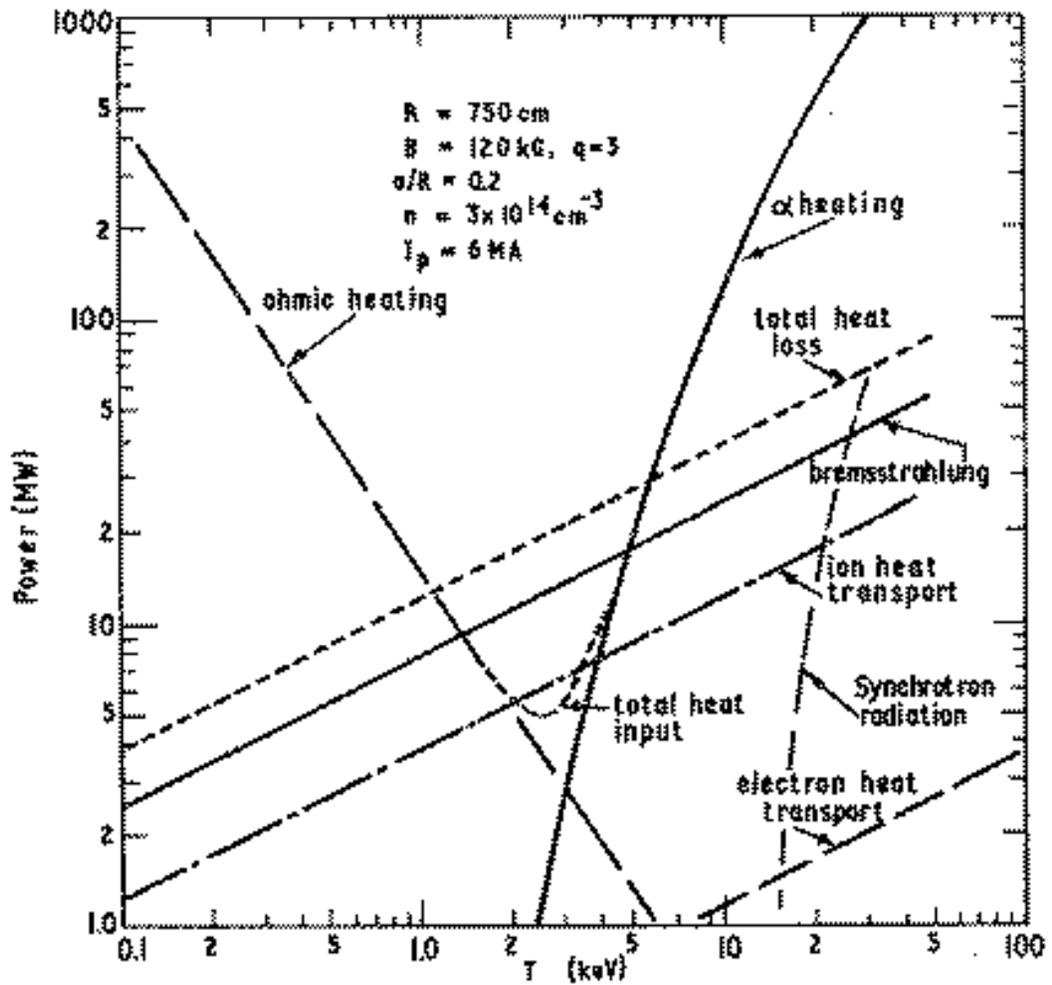
Figure 27. Energy balances in a typical Tokamak.
