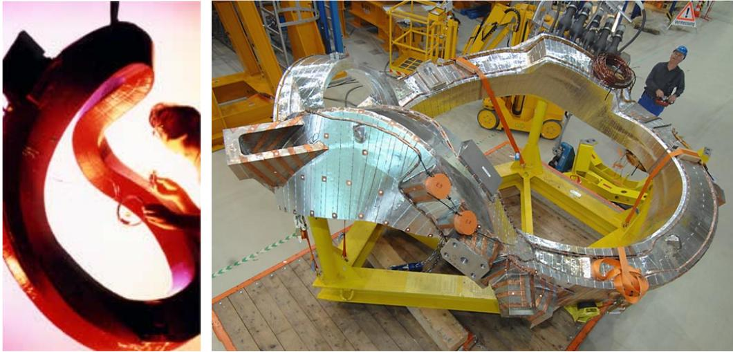
Figure 8. A single superconducting magnet coil for the 7-X Stellarator at Wendelstein, Germany.
