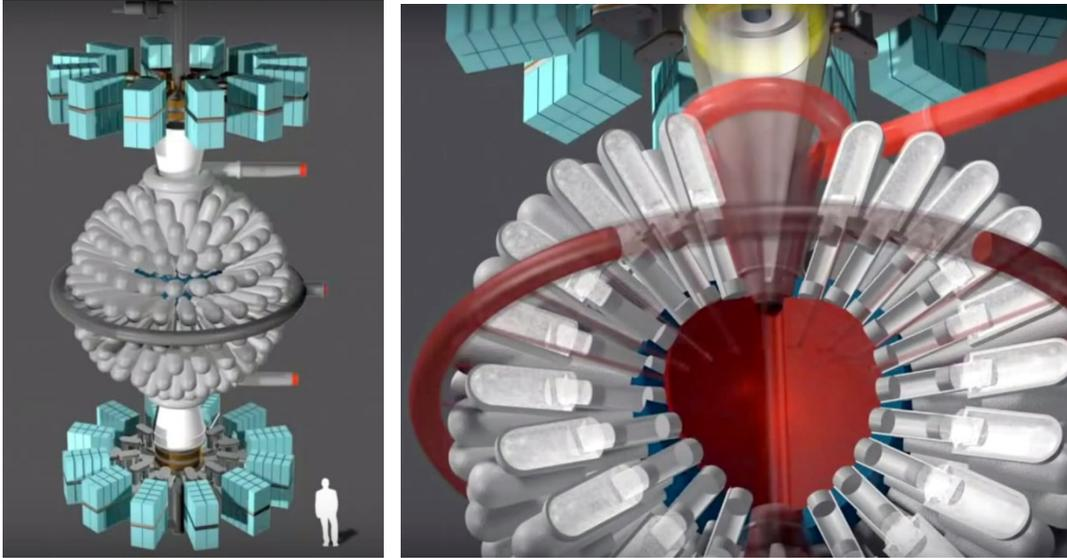
Figure 31. Magnetized target fusion reactor configuration. Liquid metal vortex is surrounded by steam-driven pistons.
