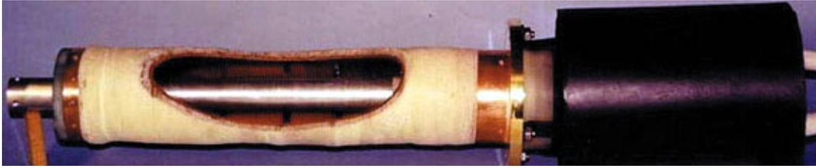
Figure 29. Magnetic flux compression generator. Aluminum tube surrounding a copper wire helix is compressed by a chemical or nuclear explosive. At the other end a transformer couples the generated current pulse to the load. Photo: LANL.
