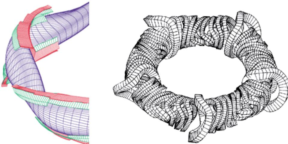
Figure 10. Divertor and coils of the 7-X Stellarator.
