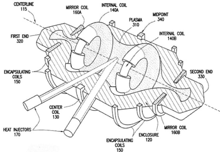
Figure 33. T4 compact high-beta conical-cusp mirror experiment. No power production or propulsion components are shown. Source: Lockheed-Martin.
