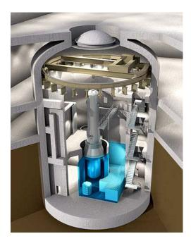
Figure 1. Schematic of modular mPower compact underground reactor. Source: Babcock & Wilcox.
