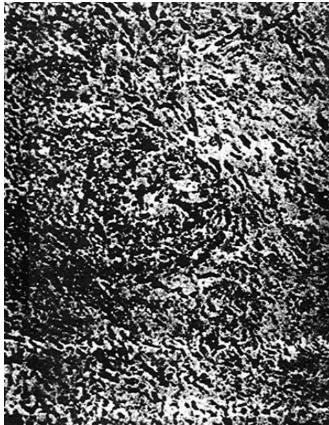
Figure 9. Sample of helical ore in a kaolinite matrix suggesting thermal effects in a clay rich in water with convective movement. Magnification is 100 times.
