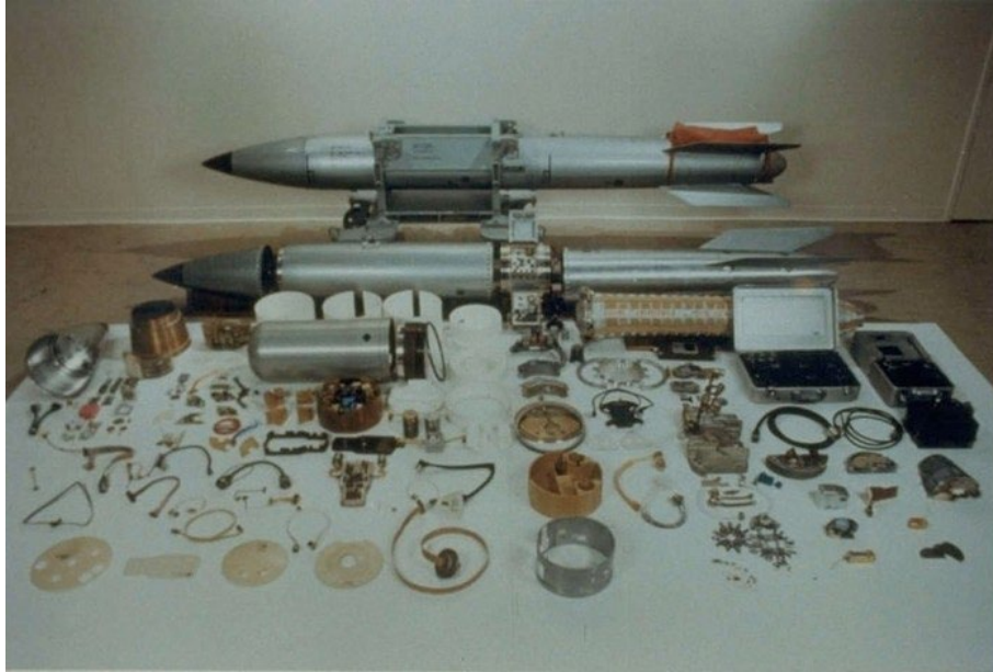
Figure 115. The B61 thermonuclear free-fall precision guided munitions with tail flaps. It is a variable "dial-a-yield" design with a yield of 0.3 to 340 kT of TNT equivalent in its various mods. The B61 is a low to intermediate-yield strategic and tactical thermonuclear gravity bomb which features a two-stage radiation implosion design. It is capable of being deployed on a range of aircraft such as the F-15E, F-16 and Tornado. It can be released at speeds up to Mach 2 and dropped from as low as 50 feet where it features a 31 second delay to allow the delivery aircraft to escape the ensuing blast wave.
