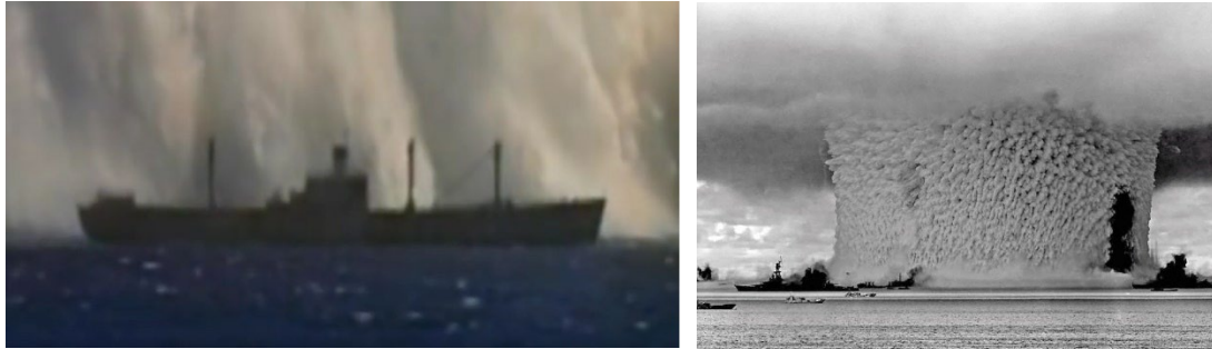
Figure 5. Crossroads under water Baker test sequence. The water column was hollow in the center and 610 meters in width. It lifted 2 million tons of sea water which created a base surge 274 meters in height and a tsunami 5 meters in height as it reached the Bikini beach 6 kms away. The Japanese battleship Nagato survived for 5 days then capsized and sun in the lagoon. Many ships could not be decontaminated and a planned third test after the Able air burst and the Baker underwater tests in the series was cancelled. Five vessels were put back into service.
