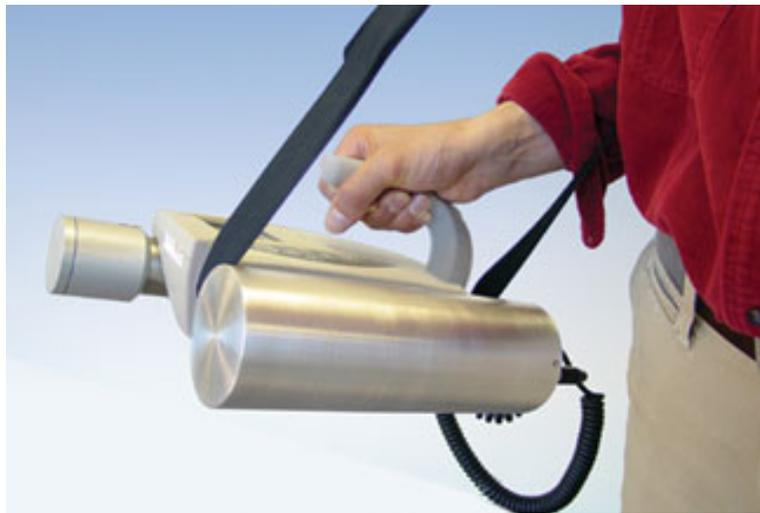
Figure 22. Hand held neutron probe.
