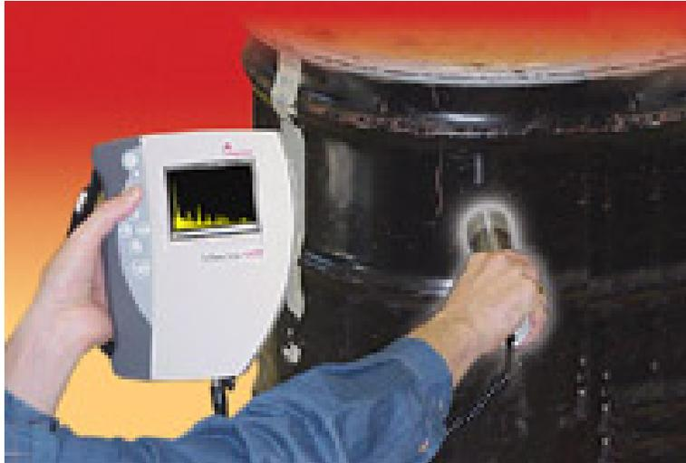
Figure 21. Hand-held identifier checks the contents of a drum.
