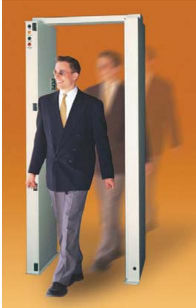
Figure 17. Pedestrian gamma and neutron monitor.
