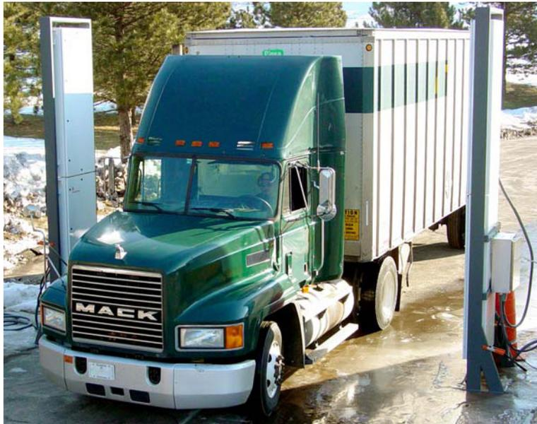
Figure 18. Special Nuclear Material (SNM) and other radio nuclides vehicle portal.
