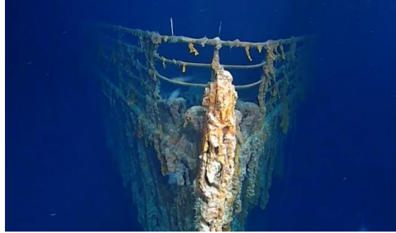
Figure 2. The use of mild steel that becomes brittle at cold temperatures contributed to the sinking of the “unsinkable” Titanic in 1912 on its maiden trip to New York and the end of the large transatlantic vessels travel with bacteria feeding on the wreck in 2019.
