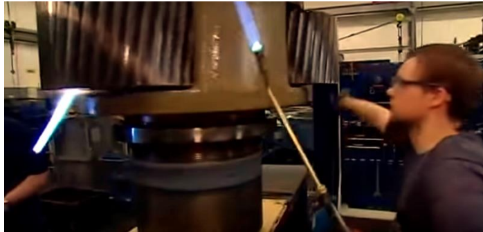
Figure 12. Overhaul of nine years old planetary transmission.
