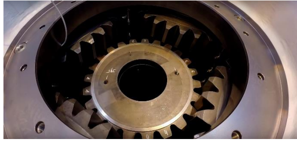
Figure 2. Wind turbine planetary transmissions during manufacture.
