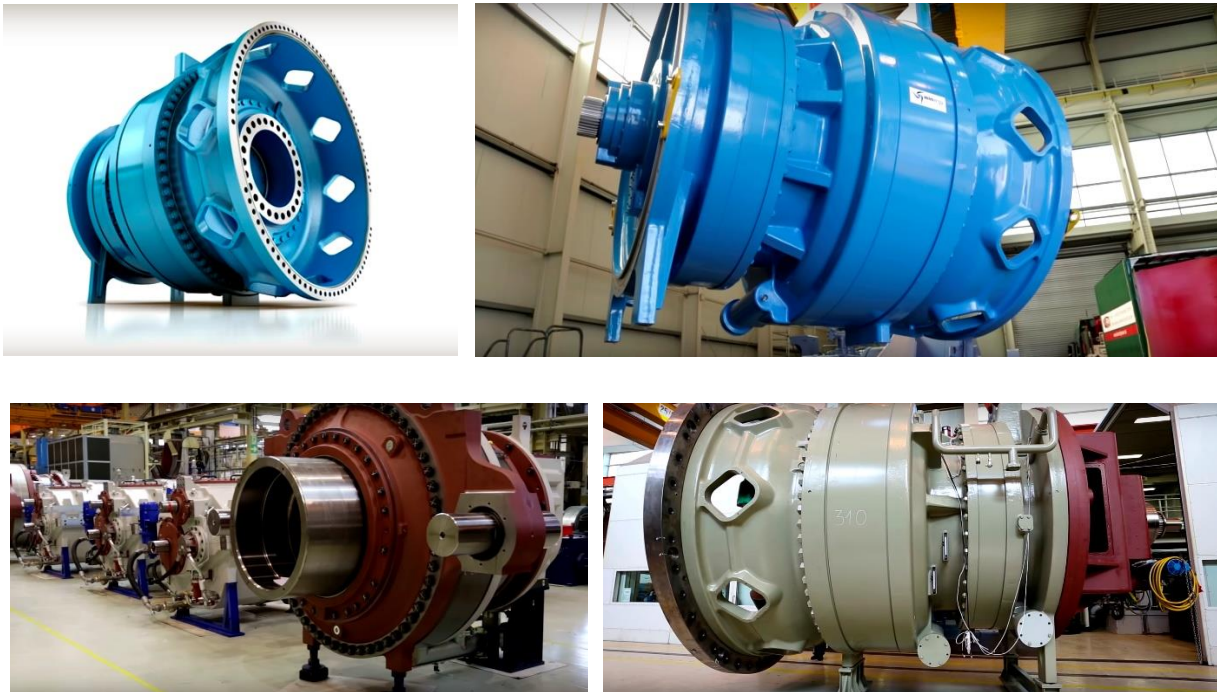
Figure 3. Assembled Winenergy 8 MW wind turbine gearbox.
