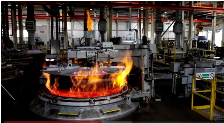
Figure 10. Gear box hardening heat treatment.
