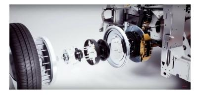
Figure .8 In-wheels independent electric motors provide an all-wheel capability.
