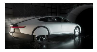
Figure 7. Lightyear wind tunnel testing.
