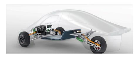
Figure 5. Composites chassis and battery emplacement.
