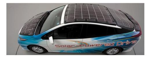
Figure 1. Toyota Solar Powered Drive Prius PHV Prime can charge its batteries while the car is driving.
