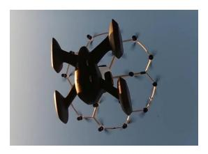
Figure 1. HEXA electric eVTOL aircraft, "flying car".
