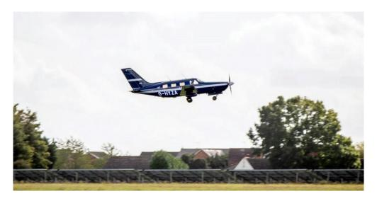
Figure 5. HyFlyer six-seater hydrogen airplane. Its successor is planned to seat up to 20 passengers. Source: ZeroAvia.
