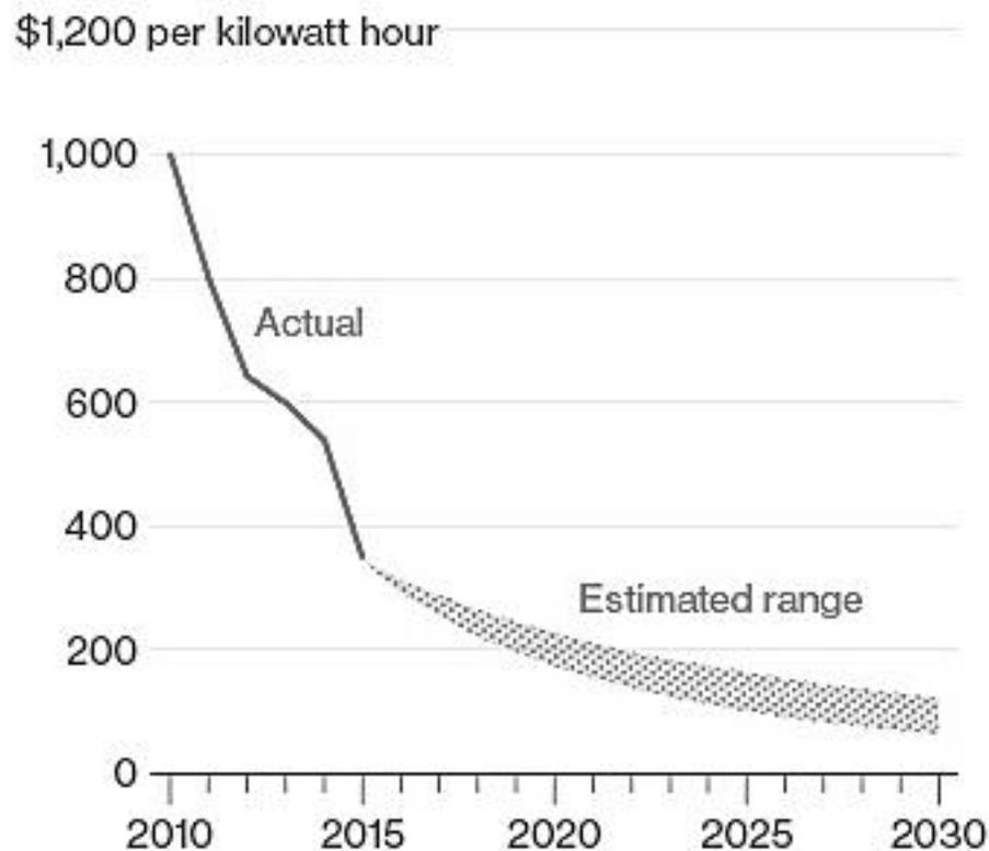
Figure 11. Price of Li-ion battery packs for electric vehicles use. Source: Bloomberg.
