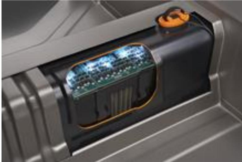
Figure 2. Lithium-ion battery pack of the Volt car. Source: GM.
