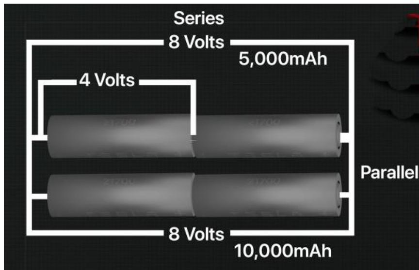
Figure 6. Tesla Cylindrical 2170 cells for battery pack is composed of 4416 lithium-ion battery cells in 16 modules wired in series for higher voltage or in parallel for higher capacity hence larger cruising range configurations.
