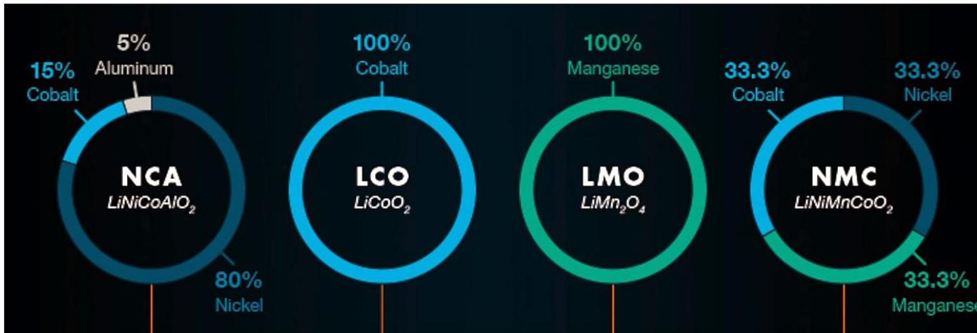
Figure 5, Types of Li ion batteries used by different car manufacturers. Li is the 25<sup>th</sup> element in abundance on earth. Aluminum, Nickel, Cobalt, and Manganese are also used.
