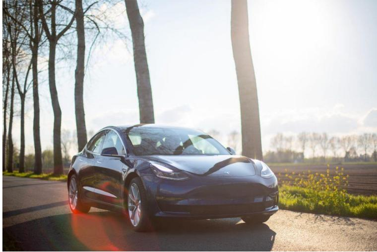
Figure 3. Aerodynamics are enhanced without need for a radiator cooling grid at the front. A lower flexible vent opening provides air flow for liquid radiator cooling. The four-wheel-drive version, with a 310-mile driving range and a premium interior, has a price out the door of \$51,000; with \$9,000 of federal and state tax credits, resulting in a net cost of \$42,000 in 2019.
