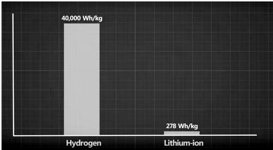
Figure 13. Comparison of specific energy content of hydrogen and lithium-ion batteries as energy storage media. Hydrogen provide a larger energy storage density capability compared with Li-ion technology. Batteries may need replacement after 2-5 years. Car range decreases after a few years of use.
