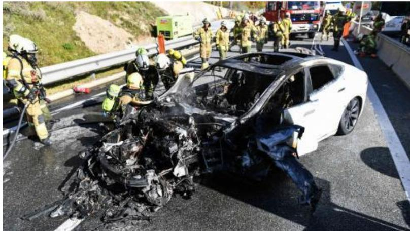
Figure 15. Tesla Li ion battery fire in Germany, 2017, suggests a need for lower risk energy storage options. According to UL Laboratories: "Lithium-ion battery technology is not intrinsically safe. Short circuit, overcharge, over-discharge, crush, and high temperature can lead to thermal runaway, fire, and explosion."
