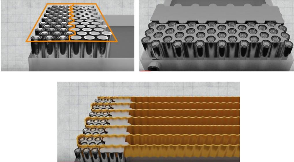
Figure 7. Battery pack bricks connected by a busbar in parallel. A cooling manifold as a ribbed interface that is a good heat conductor and good electrical insulator surrounds the cells and is cooled by a liquid water and glycol flow to a radiator.
