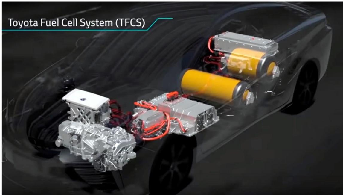
Figure 12. Toyota Fuel Cell System (TFCS) EV uses hydrogen as an energy storage medium.
