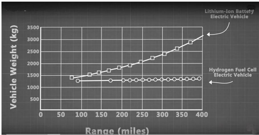
Figure 14. Comparison of vehicle weight using hydrogen fuel cell vs. Li-ion batteries. Li-ion batteries result in heavier vehicle for enhanced range.
