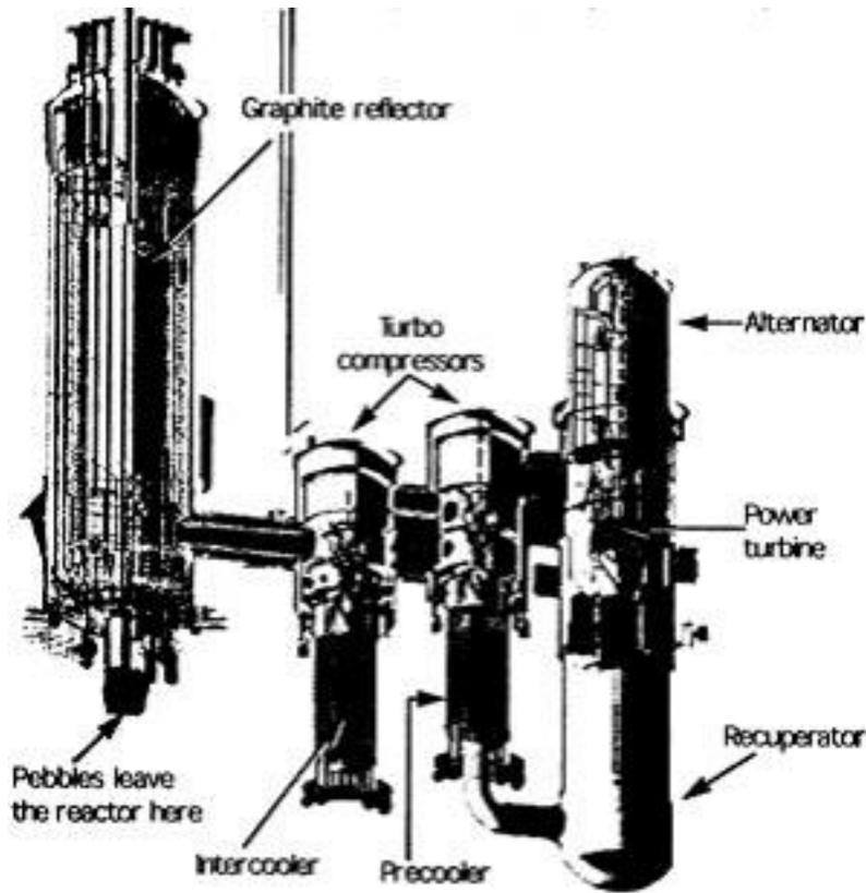
Figure 2. Diagram of the Pebble Bed Modular Reactor (PBMR).
