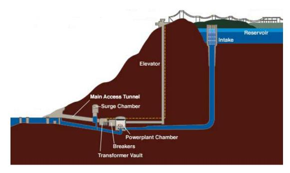
Figure 1. Pumped Storage system configuration.
