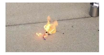
Figure 1. Li ion battery fire in air.
