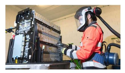
Figure 2. Safety features used in the dismantling a Renault electrical vehicle battery. Source: Olivier Guerrin.
