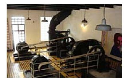
Figure 4. Electrical generators in run of river hydroelectric power.
