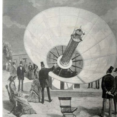
Figure 3. Truncated cone (inverted lamp shade) dish engine developed by Augustin Mouchot exhibited at the Lycée de Tours (left) and the Paris exhibition where it was used to operate an ice-maker in 1878 (right) and earned a Gold Medal.
