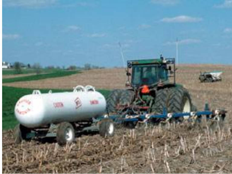
Figure 95. Tractor pulling an anhydrous ammonia applicator and liquid NH 3 tank in corn on corn ground. Photo: USDA/NRCS.
