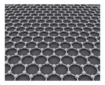
Figure 2. Graphine hexagonal cell structure.
