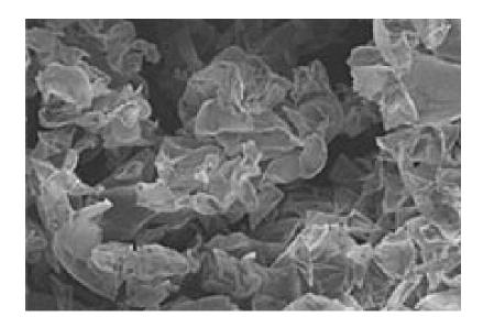
Figure 4. Crumpled graphine offer a large surface area for electrical charge storage in ultra-capacitors.
